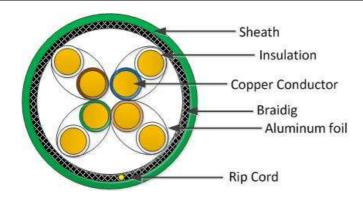
23 AWG S/FTP 4-Pairs Cat.7 Solid Wire Cable
